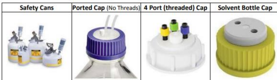
Figure 11.5b - Proper LC Waste Collection Processes
